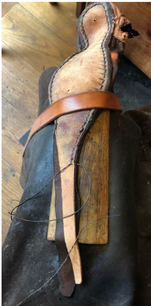
Fig. 5 The medial side of the long toe being stitched from the inside of the shoe. (Photo by M. Volken)
